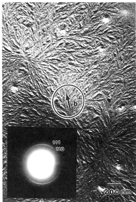
Figure 2. TEM observations of PEKK(T) spherulitic crystals grown from the melt at 180 °C for 2 h. An ED pattern is also included which is taken from the circled area in the figure and shown in correct orientation.
